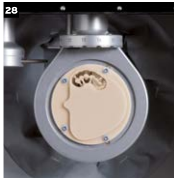
The PMMA blank with the frameworks milled in the Ceramill Motion 2.
