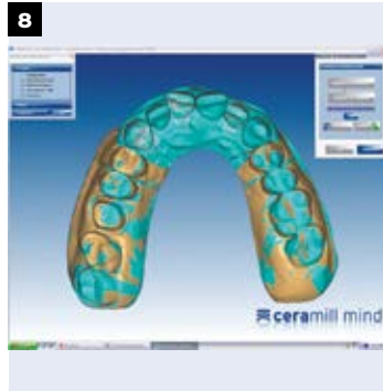
The design software (Ceramill Mind) automatically positions the diagnostic model on the residual dentition optimally.
