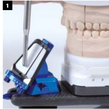
1 Setting up the incisal guidance using diagnostic models to represent the preoperative status for fabricating the anterior restoration.
