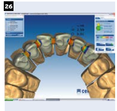
The connectors for splinting the crowns are custom-designed for the case, taking into account the minimum diameter required for the specific material.
