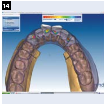
The thickness and location of those tooth regions which lead to contact areas are recognisable.
