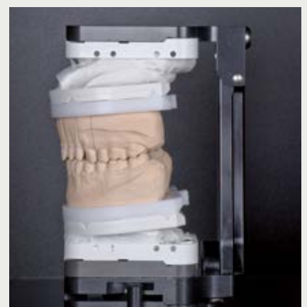
Ceramill Map400 with model in the Ceramill Fixator - for lossless transfer of the model situation.
