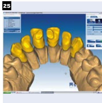
The framework is automatically reduced by the thickness required for building up the veneer. The selected guidance facets are retained.
