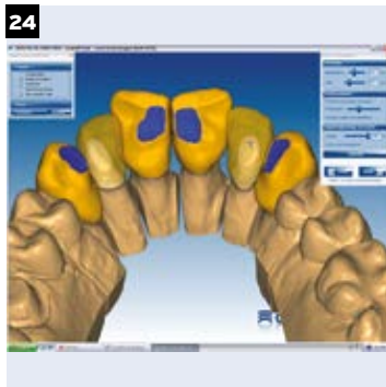
Those areas of the teeth are marked which are to be retained as guidance facets.
