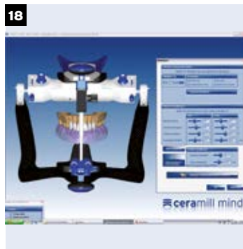
The simulated excursions are carried out using the programmed articulator parameters such as sagittal inclination of condylar guidance, Bennett angle, immediate sideshift and the custom incisal guidance table.
