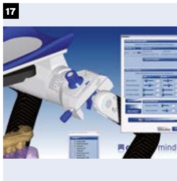
The settings are programmed by graphic animation in real-time on the Ceramill Artex. Like this, they also correspond optically to those of an actual articulator.
