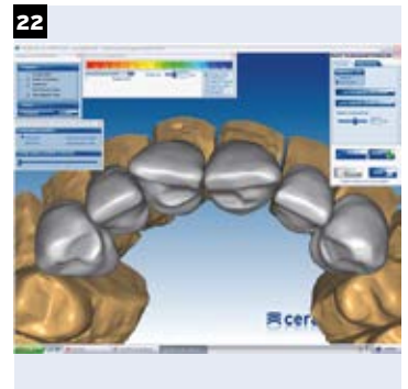
22 Any interferences or contact areas identified on the pattern during dynamic adaptation to the opposing dentition are reduced automatically.
